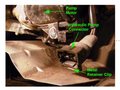
FIGURE 4 Hydraulic Pump Connector Detail
