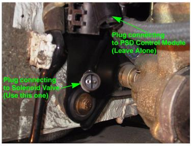
FIGURE 3 PSD Solenoid Connector
