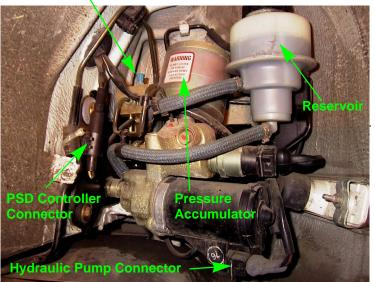
FIGURE 1 PSD Components
