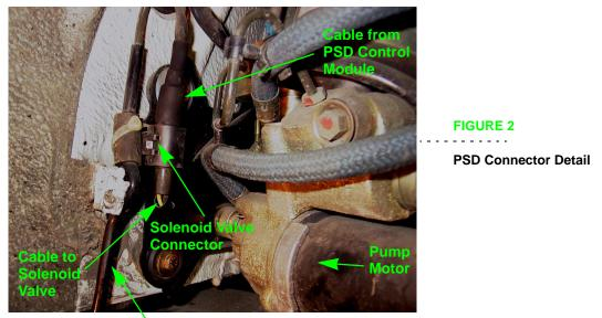
**High Pressure Line to PSD Cylinder**
