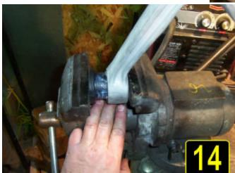
Picture #14. Put the A-Arm and a bushing in a vise and use the vise to press the bushing into the upper A-Arm.
