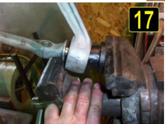
Picture #17. Use the vise and start the other side of the polyurethane bushing into position.
