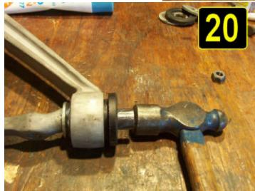
Picture #20. Tapping the center sleeve into the polyurethane bushing.
